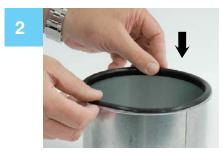
Carefully place the gasket along the rolled edge of the part, being careful to avoid kinks or voids. Only one gasket is needed per joint.
