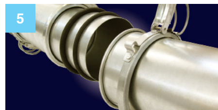
Put Adjustable Nipple O-ring on the cut pipe, then add the Oil Mist O-ring (which has a smaller thickness), and slide an Adjustable Nipple over the cut end. Seat the Oil Mist O-ring evenly and firmly against the rolled metal edge of the Adjustable Nipple. Then position the Adjustable Nipple O-ring firmly against the Oil Mist O-ring.
