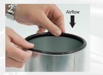
2) Carefully place the gasket along the rolled edge of the part, being careful to avoid kinks or voids. Only one gasket is needed per joint.
