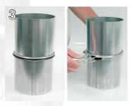
3) Join the gasketed end of the pipe to a non-gasketed end of the next part in the ducting run using a standard Q-F clamp. The oil-mist gasket, in addition to the gasket inside the Q-F clamp, provides dual protection against leakage.
